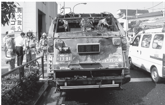
▲ Garbage truck caught on fire because of spray can
