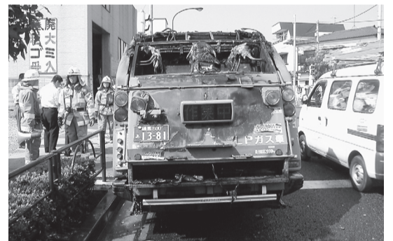
▲ Garbage truck caught on fire because of spray can
